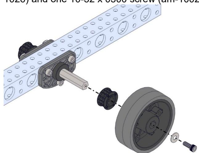
7. Place one 6mm to 375 Hex adapter (am-3444) on the NeveRest Orbital 19.2 (am-3637b) motor shaft. Make sure to secure by tightening the provided 10-32 set screw.
