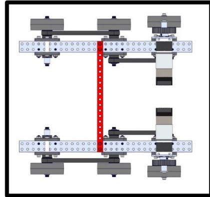
Locate one 0.5 x 0.5 x 10.0 Robits Tube (am-5001-1000) to the 2nd pair of holes from the end of the 1 inch tubes and fasten with four 10-32 x 1750 screws (am-1048) and four 10-32 nylock nuts (am-1063).
