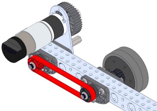
15. Slide drop mount and gearbox assembly away from the wheel to tension belt. Tighten fasteners to maintain belt tension.
