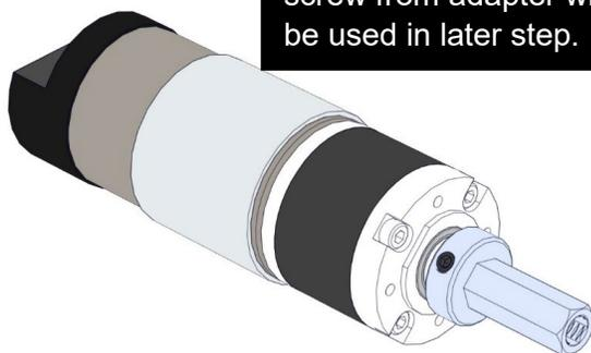
8. Attach the NeveRest motor to the three lower mounting holes on a Drop Gearbox Single Mount (am-5018\_1) using three M3-8mm patched screws (am-1500).
