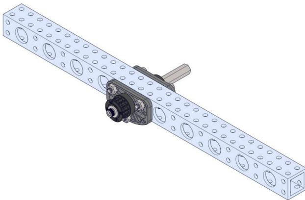
6. Install one 14 tooth pulley (am-4960) and one 3 inch stealth wheel (am-4718\_gray) to shaft and retain with one #10 washer (am-1026) and one 10-32 x 0500 screw (am-1002).
