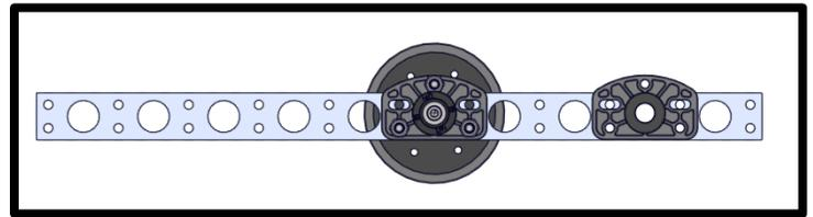
11. Turn the assembly over and loosely attach the motor and bracket through the drop mounts, tube and spacer with three 10-32 x 2000 screws (am-1049) and three 10-32 nylock nuts (am-1063). The motor should extend over the tube and be on the side of the tube opposite the drop mount spacers.
