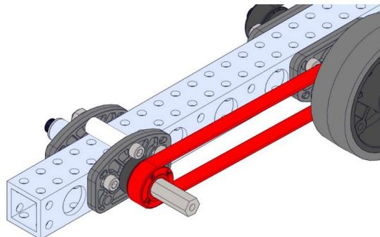
21. Slide drop mount assembly away from the wheel to tension belt. Tighten fasteners to maintain belt tension.
