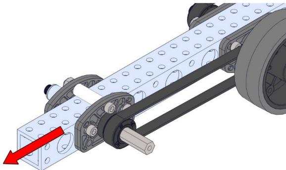
22. Add one 3 inch stealth wheel (am-4718\_gray) to the shaft and retain with one #10 washer (am-1026) and one 10-32 x 0500 screw (am-1002).
