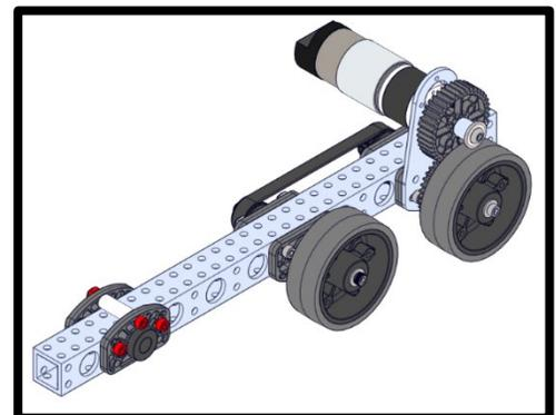
19. Fasten one 10-32 x 0500 screw (am-1002) with one #10 washer (am-1026) and one 1/2 inch shaft spacer (am-1699) to the end of a 4 inch Robits shaft (am-5003-0400).
