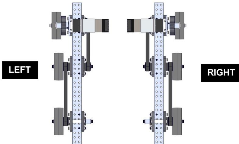
1. Insert one bushing (am-5021) into a Drop Mount (am-5019). Repeat this to create six drop mount assemblies.
