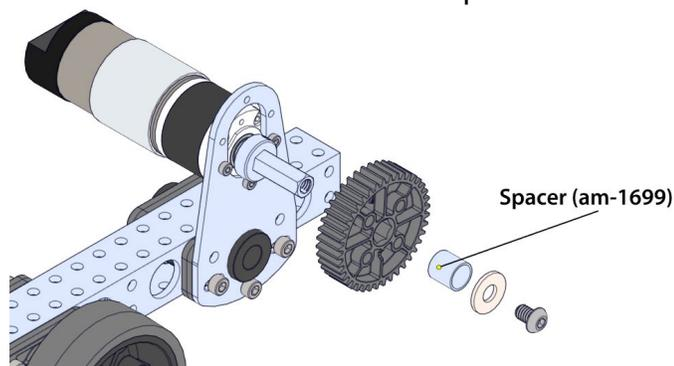
13. Fasten one 10-32 x 0500 screw (am-1002) and one #10 washer (am-1026) to the end of a 4 inch Robits shaft (am-5003-0400).
