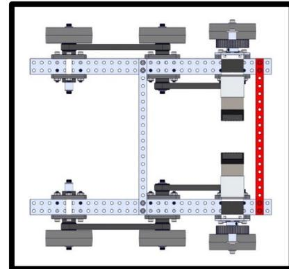
The Robits 6WD Drive Base is Complete! Use this as a starting point and add on other parts, mechanisms, and electronics to create a complete robot.
